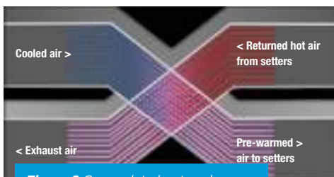
Figure 2 Cross plate heat exchanger.
